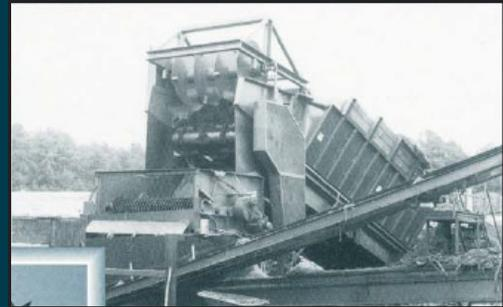
The 858 Bulk Feeder is one of three models designed to meter the flow of materials being conveyed to a particular processing line. The 440 Disc Separator mounted at the discharge point provides the initial separation of unwanted or oversize objects.
