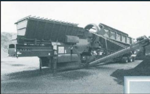
Look to Amadas Industries for a variety of screening applications where mobility is important. Our totally self-contained Portable Trommel features multi-product capability, overhead return conveyors, and maximum throughput efficiency.
