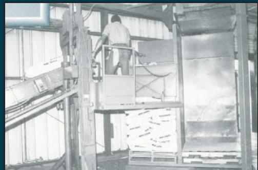
The Model 271 Semi-automated Palletizer from Amadas makes palletizing a cinch. Proper bag presentation from the conveyor to the stacker, together with an elevating platform which rises with the pallet height, allow bags to be easily received and stacked at waist level. Once stacked, the four-pallet indexing turntable revolves to the next loading screen.
