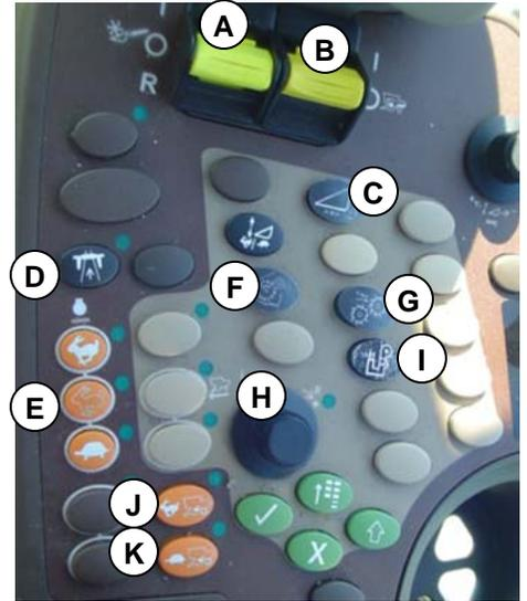
**J K 4WD** Press J to use 4WD with higher speeds. Press K to use when more traction is needed. Light indicates when in use; press again to take out of 4WD.
